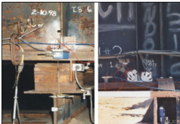
Exhibit 2. Instrumentation at Crack Locations
