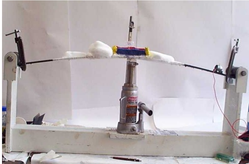
Figure 2. Photo of the bar at high deflection
